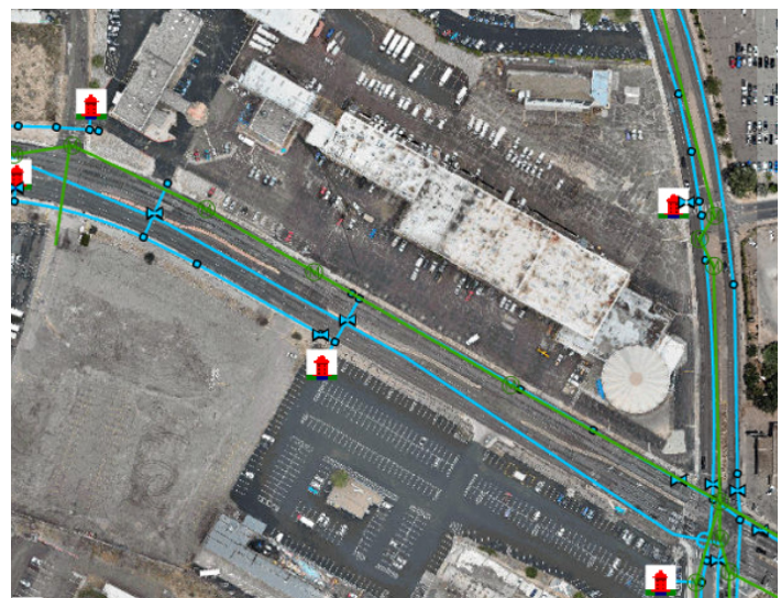
EXISTING SANITARY SEWER AND WATER LINES
