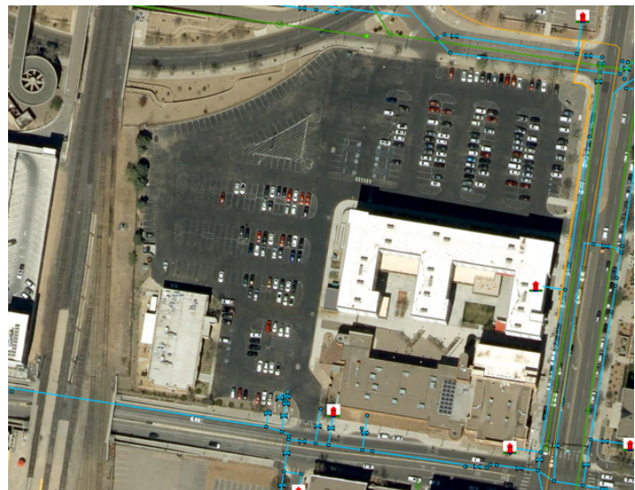
EXISTING SANITARY SEWER AND WATER LINES
